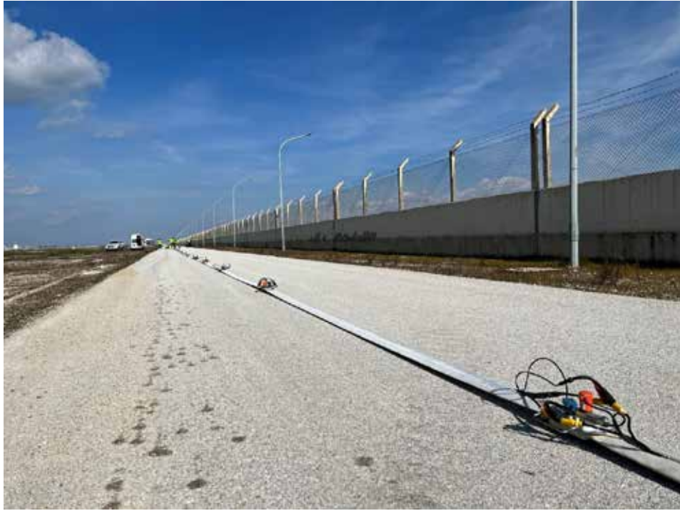
Mobile Seismic Receiver Array Measurement System developed by TÜBİTAK MAM Earth Sciences Research Group for rapid measurement in earthquake zones.
